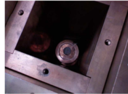
Enriched Ge sample activated at GEANIE, and counted on low-background Ge detector at WIPP.
